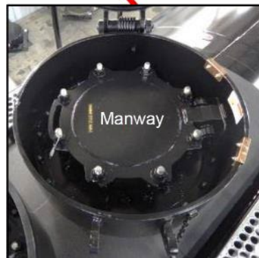
Manway with hinged and bolted manway cover
