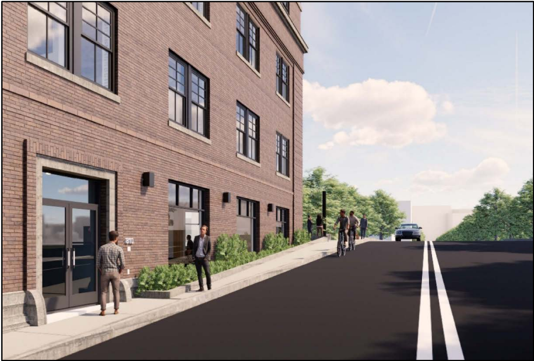
Figure 4-26: Rendering of proposed grade-separated planters fronting the former International Harvester Building at 810-822 W. North Avenue, which is designed to minimize changes to the stone foundation and minimize the visual and physical effects of the sidewalk grade change on building's façade.
